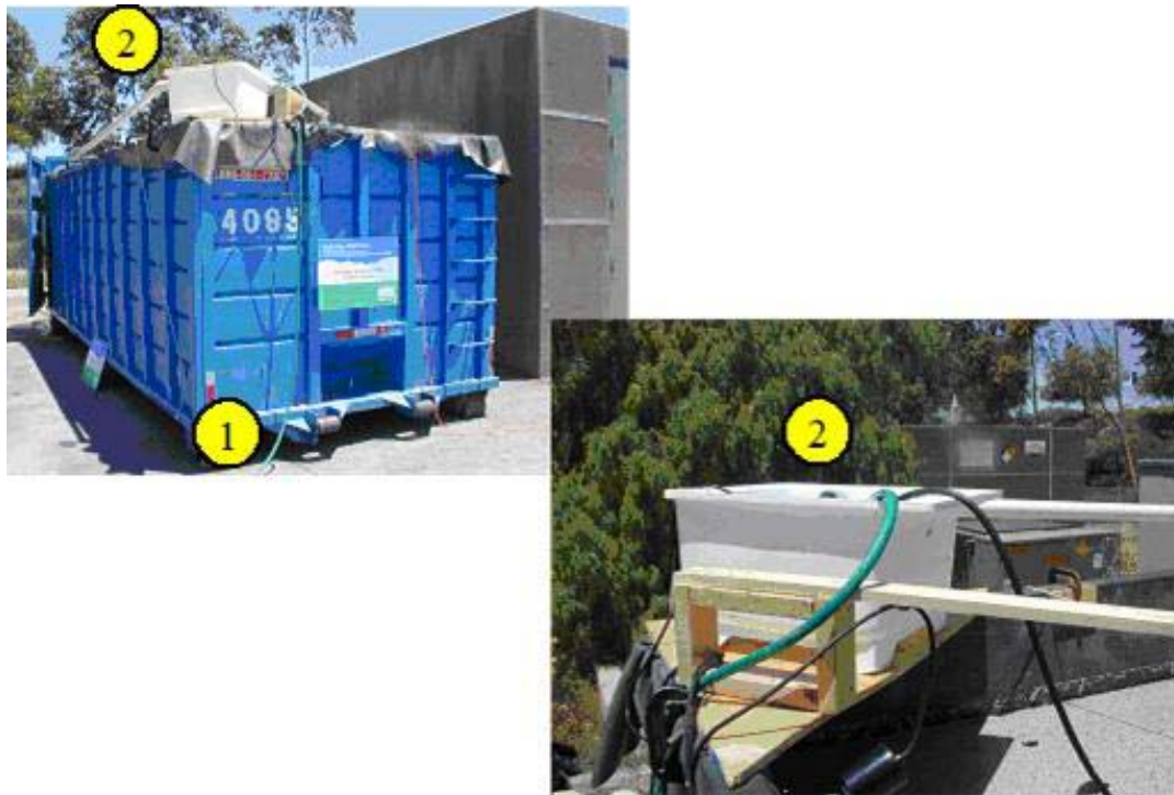
Figure 10: Source water (1) was pumped into a metering tank above the BMP (2).
